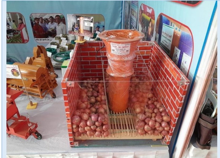
A model onion blower made by RK Metal of Faridpur, on display at the SME fair, Faridpur. The model shows the use of bamboo flooring to increase the flow of air through the onion store. May 20, 2024. Photo: Diponkor Gosh, RK Metal, Faridpur
