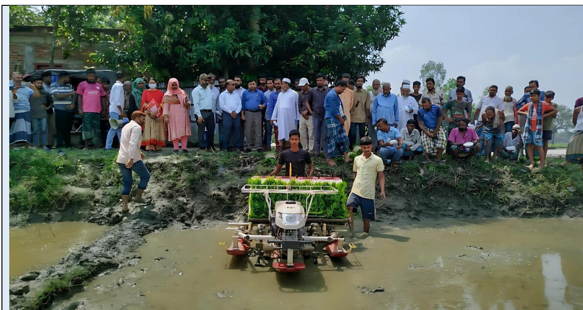
A rice transplanter MSP from Cox's Bazar, transplanting rice in Chauddagam upazila , Cumilla District, as part of the flood response activities facilitated by CSISA–MEA with USAID support. September, 2023
