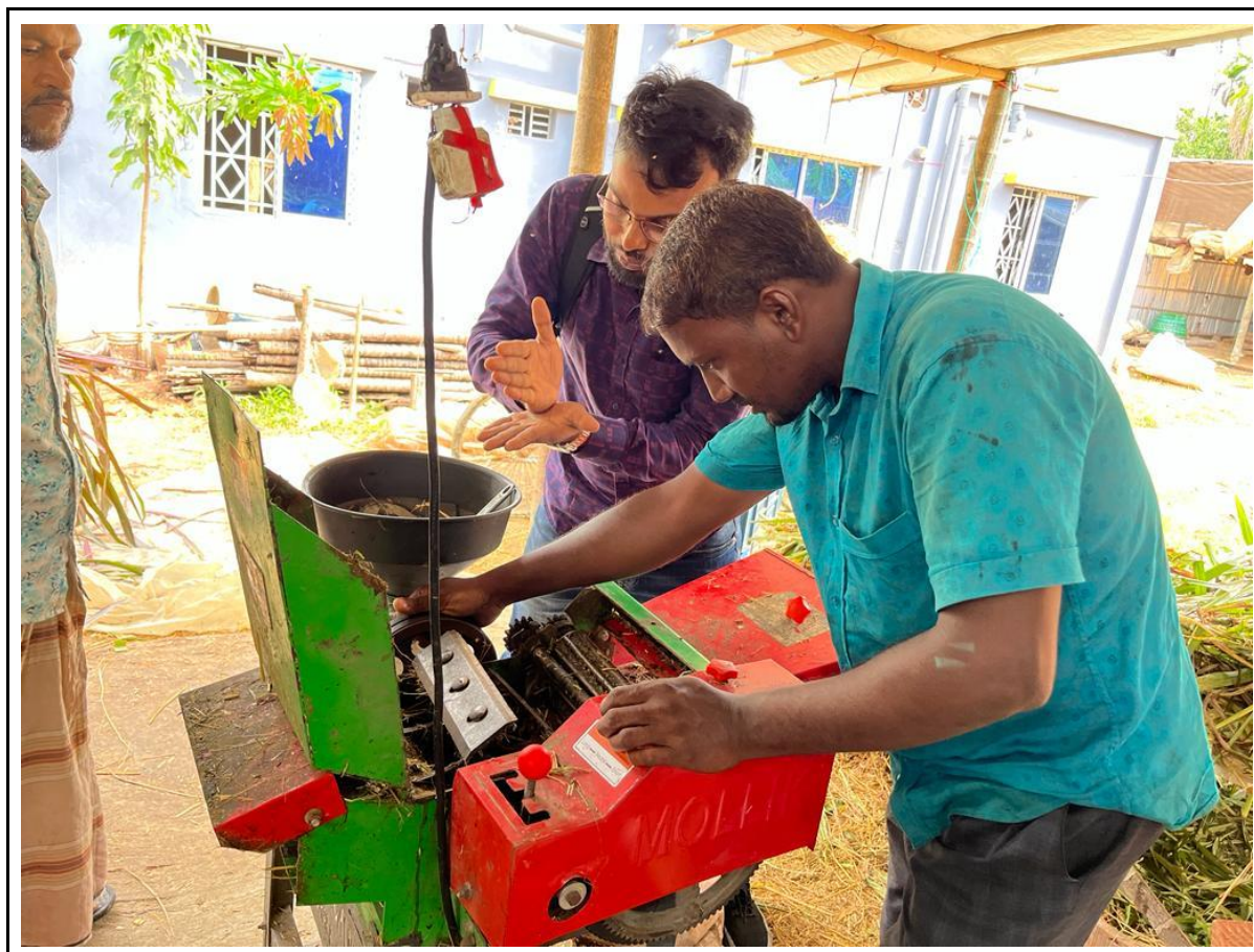
A CSISA–MEA engineer explaining the modifications needed to improve the performance of a fodder chopper manufactured by Mr. Md. Alauddin, owner of MAA Machinery Workshop, Ramu Bypass intersection, Ramu, Cox’s Bazar. November, 18 2023 Photo: Mohammad Shahidul Islam, ADO, Cox’s Bazar.
