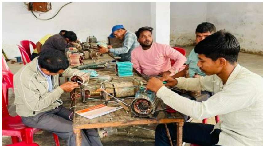
Above: pump set mechanics repairing electric motors during intensive technical training. Nepalgunj 19, Banke district. March 2024. Photo: Shreya Malla
