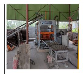
Equipment to manufacture cement blocks using slag at ZH Star Bricks, Bogura. Photo credit: J. Colton, Professor, Georgia Tech, USA
