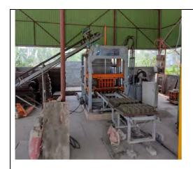
Equipment to manufacture cement blocks using slag at ZH Star Bricks, Bogura. Photo credit: J. Colton, Professor, Georgia Tech, USA
