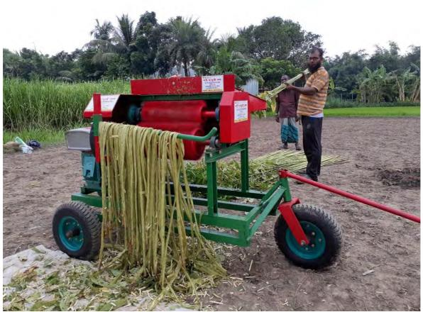
The newly developed small version of the Aashkol jute fiber extraction machine manufactured by RK Metal, being used by an MSP, Faridpur district.
