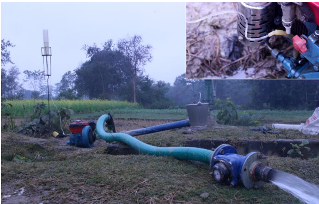
Above: Setup of pump testing rig during one of the 116 in-situ irrigation tests conducted as part of the CSISA study published in Agricultural Water Management journal . Inset image shows a close-up view of the fuel injection from the graduated measuring cylinder into the pump engine. Photo: Subash Adikhari.
