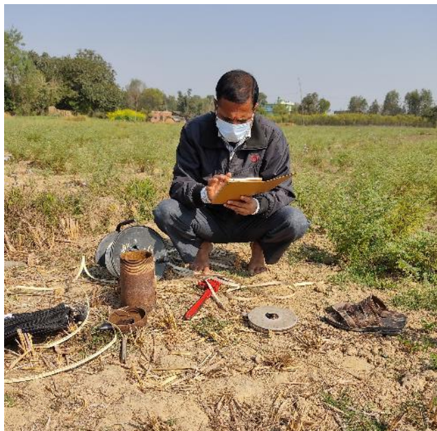
Above: Installing an offline data logger for groundwater level monitoring in Bardiya, Nepal. Photo credit: Anton Urfels.
