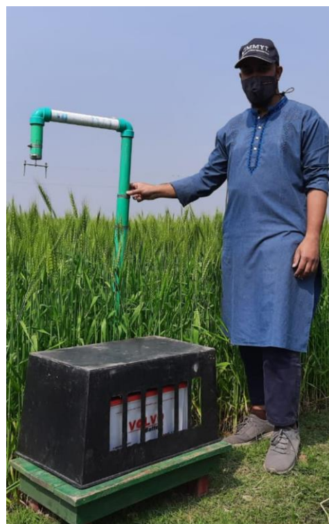
Above: Md. Harun-Or-Rashid of the CSISA team monitors wheat blast spores caught by an automatic aerial spore trapper each year to help assess the risk of wheat blast outbreak reoccurrence in Bangladesh..
