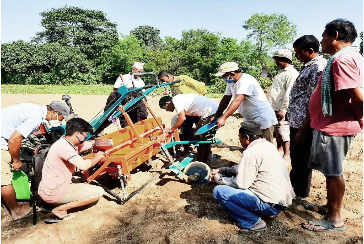
Above: Power tiller owners participating in training to operate and calibrate a two-wheel tractor operated seed drill, Harit Kranti Custom Hiring Center supported by PMAMP, Dang. (Photo: Sagar Kafle/CSISA)
