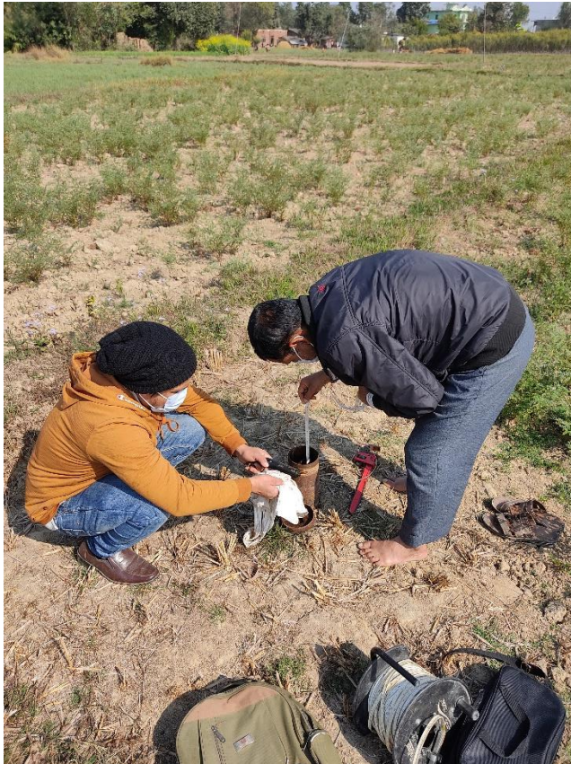
Above: Installing an offline data logger for groundwater level monitoring.
