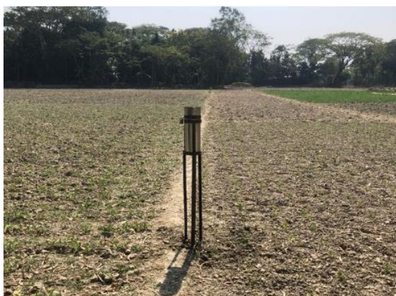
Above: 52 rain gauges like the one pictured have been installed in mung bean fields to collect rainfall data during the harvest (7 March to 7 June, 2021). (Photo: Golam Morshed Rokon/CSISA)
