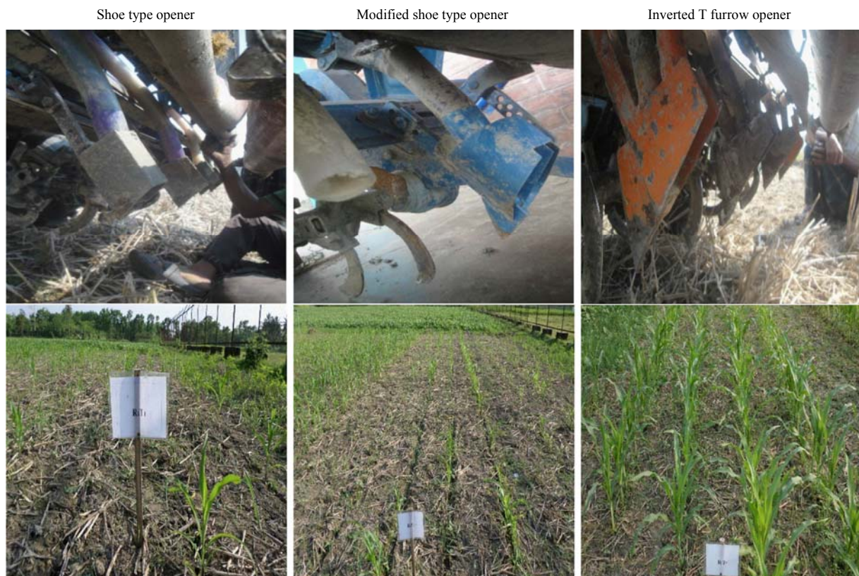
Figure 4 Types of furrow opener type and their respective crop establishment performance
