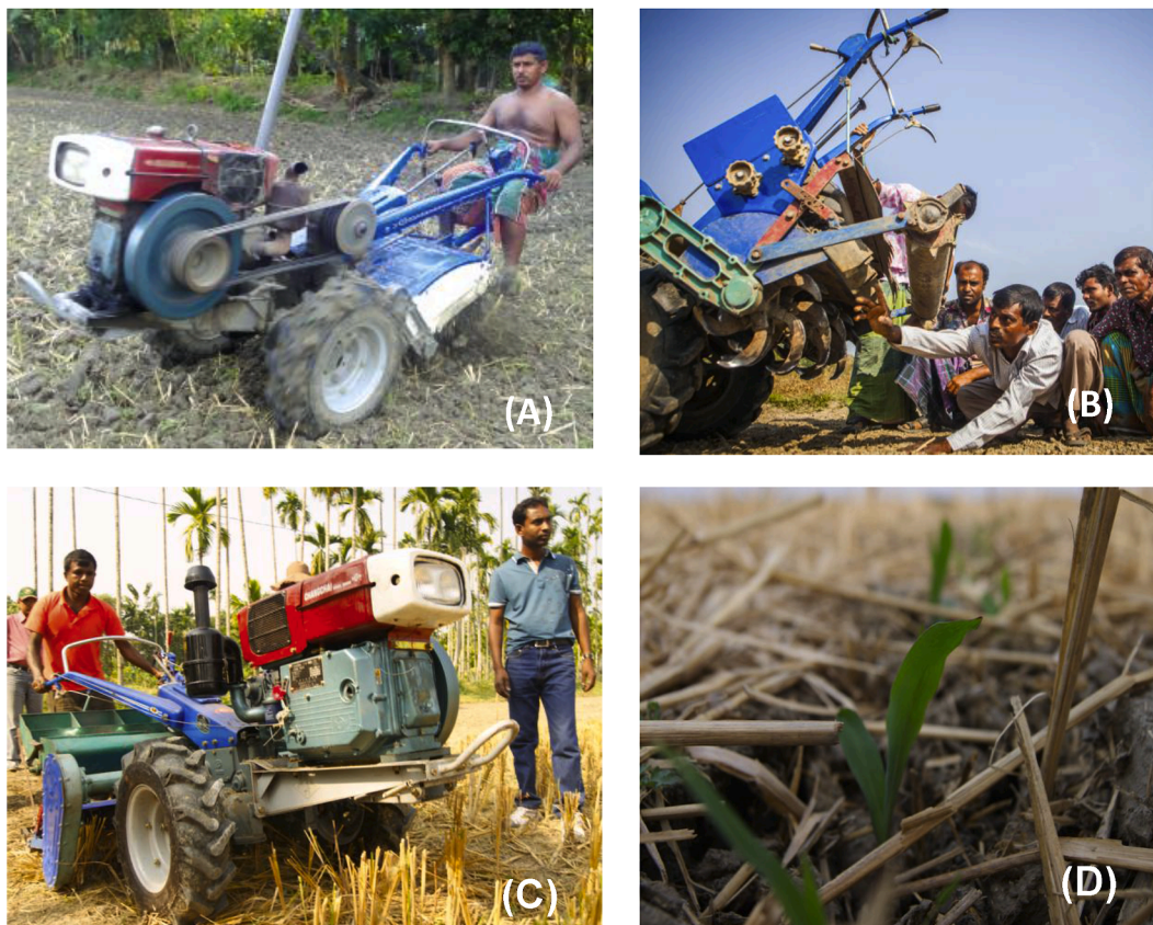
Fig. 1. (A) A Chinese manufactured two-wheel tractor power tiller used for conventional tillage in Bangladesh. (B) Detail of farmers examining the rear portion of a power-tiller operated seeder (PTOS) with conventional C-shaped blades in Bangladesh. (C) A PTOS attached to a two-wheel tractor being used to seed maize by strip tillage (note the anchored rice residue). (D) The resulting emerging maize crop. Photo A and B by R. Martin. Photos B and C by TJ Krupnik.
