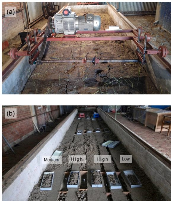
Fig. 2. (a) Soil bin apparatus and rotary axle shown with blade holders prior to experimentation, and (b) depiction of furrow backfill, soil tillage and other furrow data collection in the soil bin after test runs.
