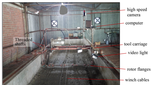
Fig. 3. Tillage test rig at the Farm Machinery and Postharvest Process Engineering Division at the Bangladesh Agricultural Research Institute, Gazipur, Bangladesh.
