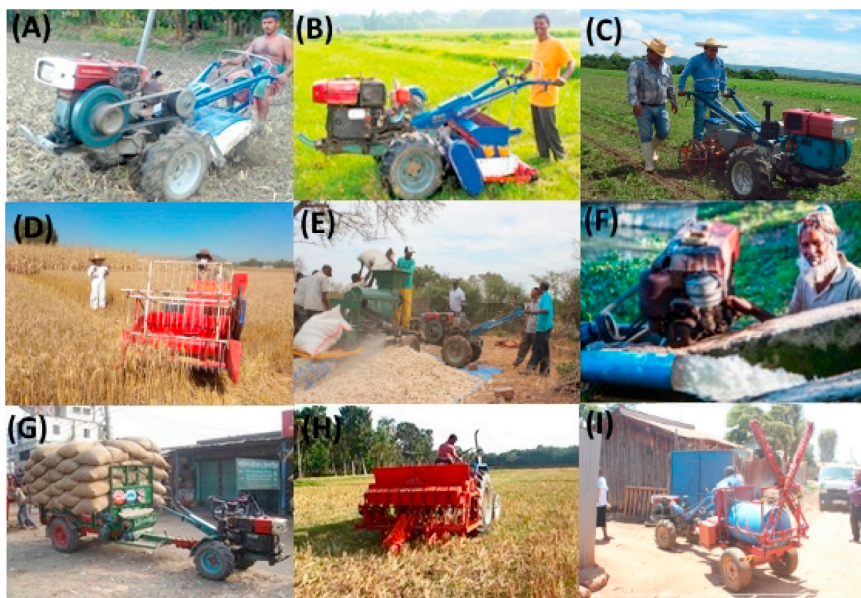
Fig. 1. Selected “appropriate” agricultural machineries used in the context of smallholder agriculture: (A) two-wheeled tractor and the removable power tiller, (B) two-wheeled tractor driven direct seed and fertilizer drill, (C) two-wheeled tractor single row planter, (D) self-propelled rice and wheat reaper, (E) two-wheeled tractor propelled stationary maize sheller, (F) axial flow pump powered by a two-wheeled tractor, (G) two-wheeled tractor trailer used to haul agricultural produce to the market, (H) “Happy Seeder” used to drill seed into rice residue without tillage, (I) small-scale sprayer cart (Photos: T. Krupnik, Md. A. Matin, S. Justice, R. Martin, A. Haque, F. Baudron, J. López).
