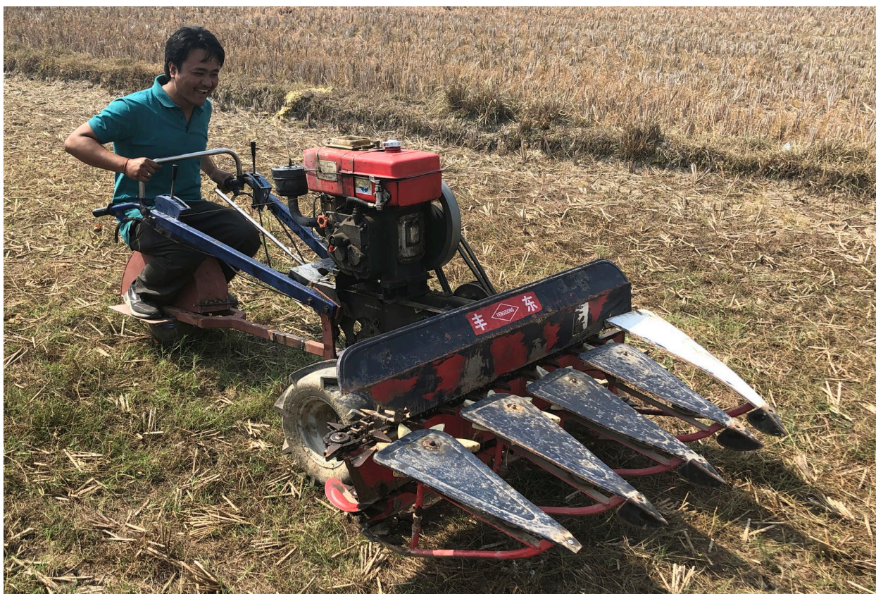
Photo 5.5: Sulky being tested for the first time in field in Bhairahawa. Note that a lesson from this test was that further modifications are needed for the comfort of the operator (Timothy J. Krupnik)
