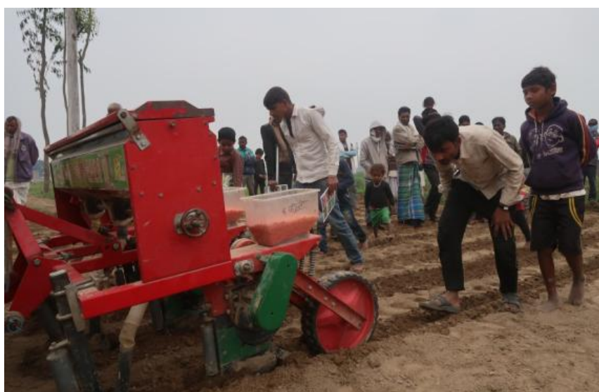
Photo 5.6: A four-wheel tractor with the 2BMZJ-3 Chinese-made precision multi-crop planter sowing maize (Hari Prasad Acharya, CIMMYT)
