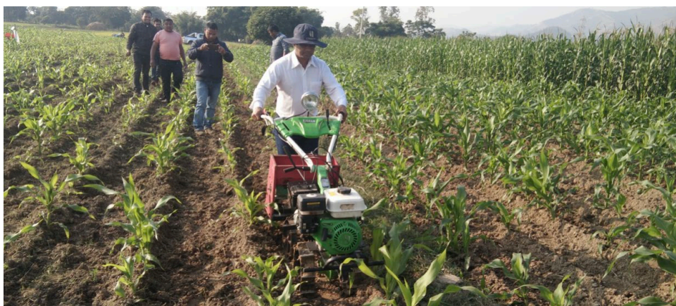
Photo 5.4: Field testing mini-tiller side-dressing attachment for maize in Dang. Preliminary evaluations indicate that this attachment can dramatically increase the efficiency of inter-cultural operations for (Hari Prasad Acharya)
