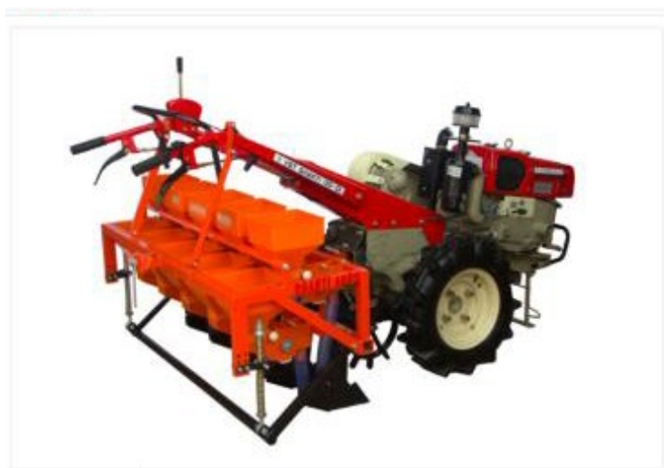
Figure 5.6: The improved Dharti 2WT seeder planter with a new easily adjustable integrated row unit is now being sold online and by machinery dealers in Nepal (Dharti)
