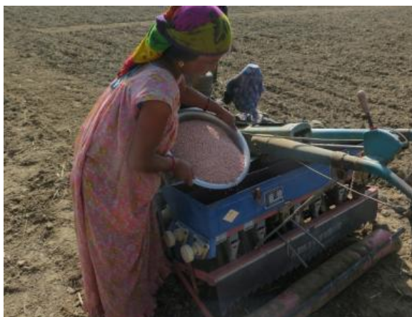
Photo 2.12: A farmer places seed in the hopper of a two-wheel tractor operated mechanical seed drill prior to line sowing by a service provider in Kailali, Nepal (Pradip Chaudhary/CIMMYT)
