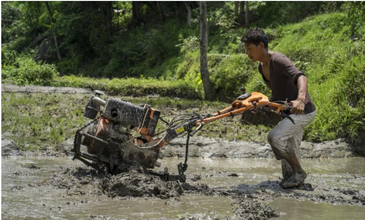
Photo 5.1: A service provider preparing a small terraced field in Nepal's Midhills with a mini-tiller for planting rice. Larger machinery is not feasible in this environment, and so the project has focused on expanding markets for scale-appropriate machinery like mini-tillers (Peter Lowe, CIMMYT)
