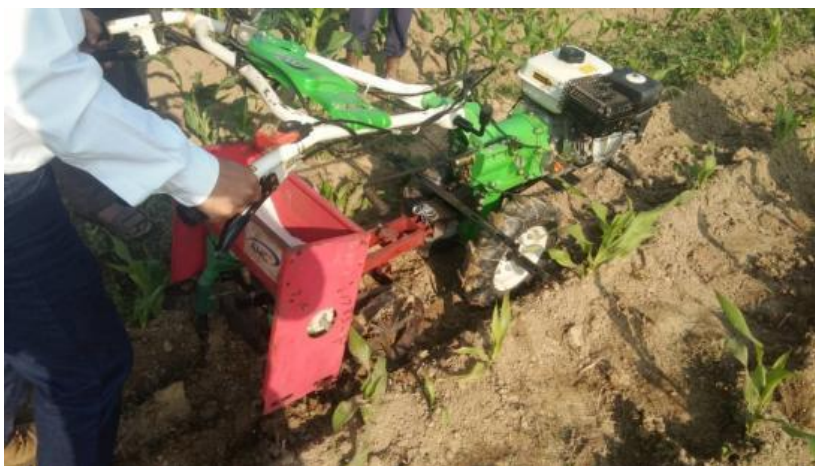
Photo 5.4: Field testing mini-tiller side-dressing attachment for maize in Dang. Preliminary evaluations indicate that this attachment can dramatically increase the efficiency of inter-cultural operations for maize farmers. (Hari Prasad Acharya, CIMMYT)
