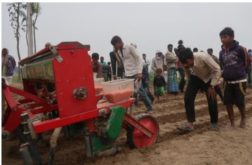
Photo 5.6: A four-wheel tractor with the 2BMZJ-3 Chinese-made precision multi-crop planter sowing maize (Hari Prasad Acharya, CIMMYT)
