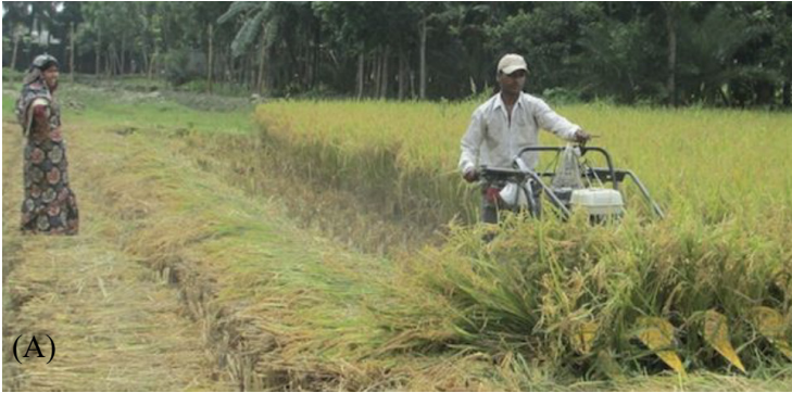
Figure 1. (A) A self-propelled reaper harvesting rice and (B) a two-wheel tractor attachable reaper, also harvesting rice in Bangladesh.
