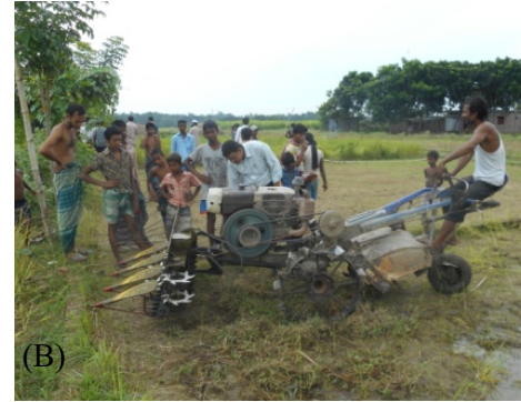
Figure 1. (A) A self-propelled reaper harvesting rice and (B) a two-wheel tractor attachable reaper, also harvesting rice in Bangladesh.
