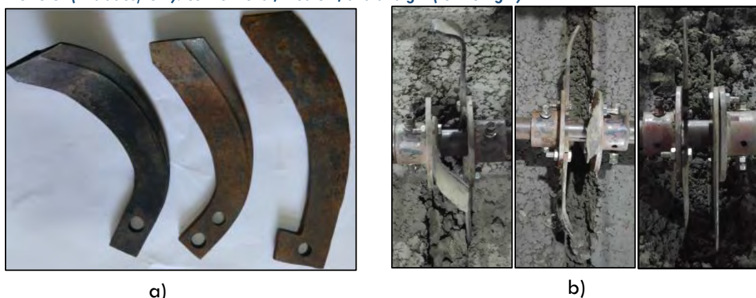
Figure 19: (a) Blades tested: conventional, medium, and straight (left to right); b) Setting of the blades on the rotor (4 blades/row): conventional, medium, and straight (left to right)
