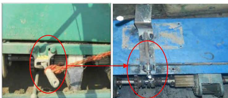
Figure 22: Replacement of the Chinese type seed on-off clutch by a simplified dog type clutch. Left - Chinese type seed on-off clutch, right - simplified dog type clutch. This modification will cost about US$ 9.00 per PTOS (parts and mechanic charge)
