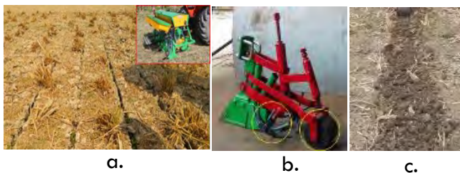
Figure 26: Design and development of press wheels for 4WT Zero-till drill to cover the seed furrow slots with loose soil. a) Uncovered slots left by the ZT furrow openers causing poor germination and plant growth, b) furrow opener (painted in greens) fitted with the press wheels (parts circled and painted in reds), and c) nicely covered slots left by the furrow opener when fitted with the press wheels.
