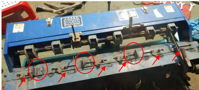
Figure 25: The existing furrow opener clamps (marked with arrows) on the ACI model PTOS do not allow enough adjustment to obtain 300 mm row spacing required for mung bean or other crops sown on a 300 mm row. Therefore, three additional clamps (marked with circles) are welded beside the existing clamps to allow sowing crops on a 300 mm row spacing. Cost of modification is about US $ 2.5/PTOS (parts and mechanics charge)
