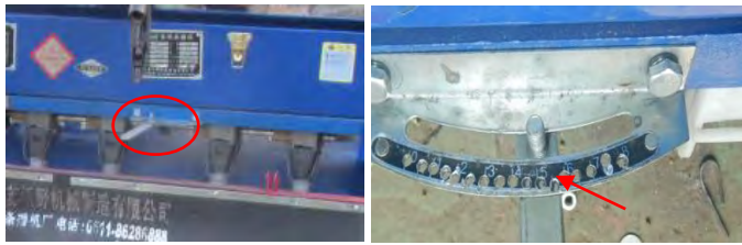
Figure 24: Modification of the seed meter control lever locking mechanism on the PTOS. Left – existing seed metering control lever with in appropriate locking mechanism, which easily slips thus altering the seed rate. Right – improved locking mechanism (2 mm hole and a pin lock- slip proof). Cost of modification is about US $ 2/PTOS (parts and mechanics charge)
