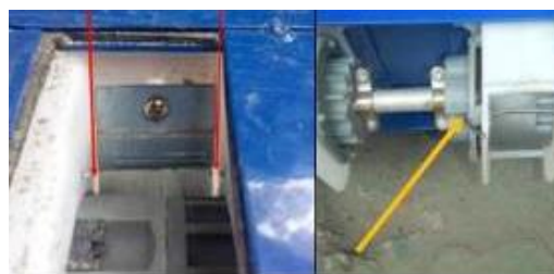
Figure 17: The existing nylon brush inside the seed box (a) is replaced a metal tongue (b) to correctly meter the seed as per calibration
