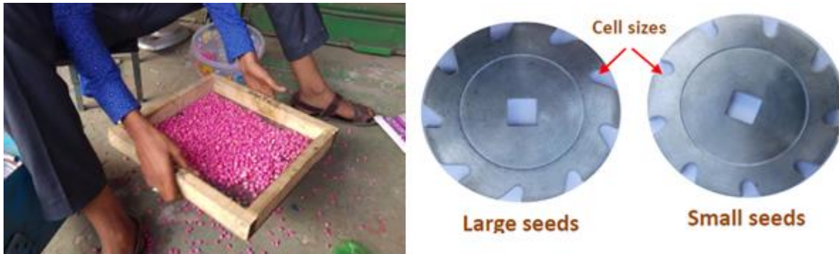
Figure 18: a. Grading treated maize seed in to large and small seed lots, and b. the modified inclined metering plate for large and small seeds
