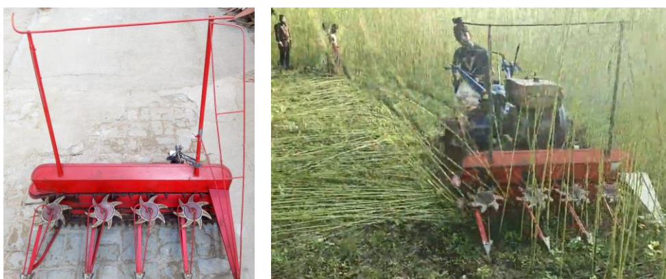
Figure 21: Modifications to the 2WT attached reaper to harvest jute
