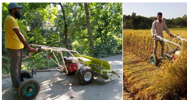
Figure 22: Newly developed Sulky wheel for self-propelled reaper transportation. Photo: Belal/ CSISA MI
