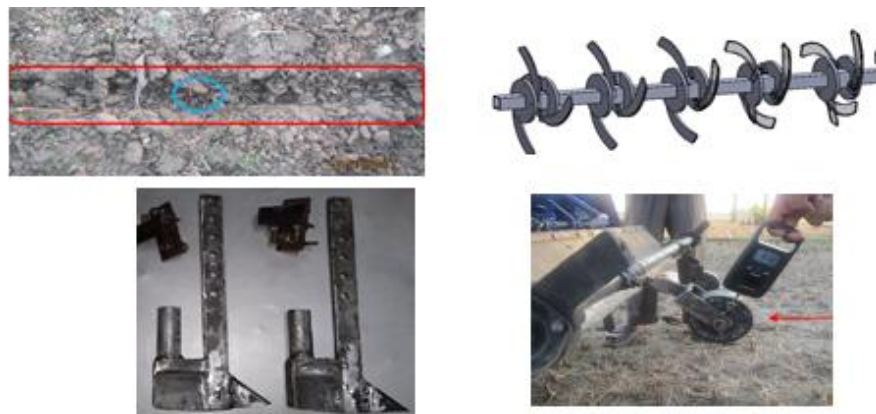
Figure 19: (a) Exposed seed in the furrow due to poor backfill, (b) Redesigned rotor and straight blades, (c) Modified openers to reduce slot width and depth control, (d) individual press wheels to follow soil terrain and provided soil seed contact
