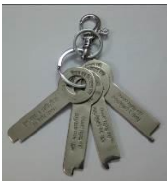
Figure 15: The Stainless steel Calibration Keys for adjusting seed rate for fluted roller seed meters for wheat, lentil, mung bean and jute
