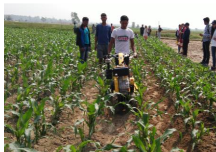
DEMONSTRATION AND TRAINING OF MINI-TILLER MODIFIED INTO POWER WEEDER FOR WEED MANAGEMENT AND EARTHING UP IN MAIZE IN DANG
