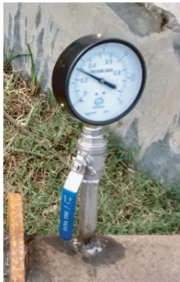
Figure 4: Pressure Gauge connected to ball valve
