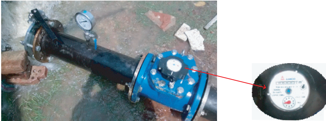
Figure 3: A Woltman Flow Meter installed for pump testing. Note that the discharge point of the pump is located to the lower right side of the meter. For normal pumping operations, the flow meter (blue colored) and all to the left would not be present.
