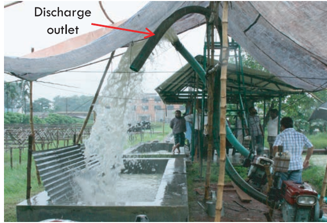
Figure 13: Pump Testing at BARI by raising the discharge outlet of the pumping system.
