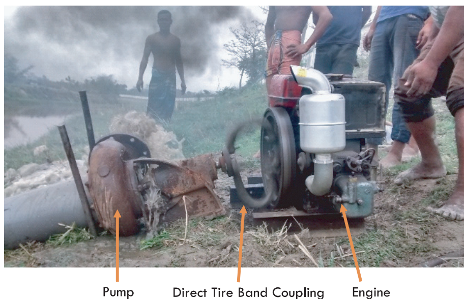
Figure 7: Direct Tire Band Power Couplings on a Centrifugal Pump
