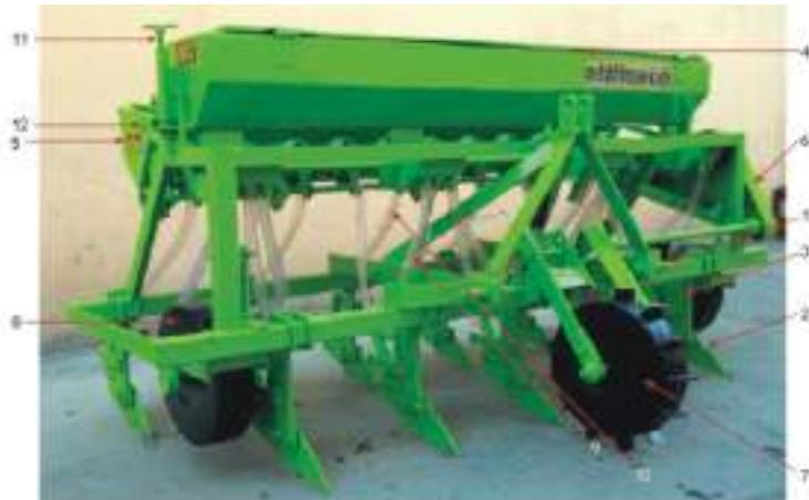
1. Frame, 2. Fertilizer spreader, 3. Tines, 4. Fertilizer box, 5. Seed box, 6. Chain and gear drives, 7. Drive wheel, 8. Depth control wheel, 9. Fertilizer delivery pipe, 10. Seed pipe, 11. Fertilizer rate adjusting nut, 12. Seed rate adjusting step.
