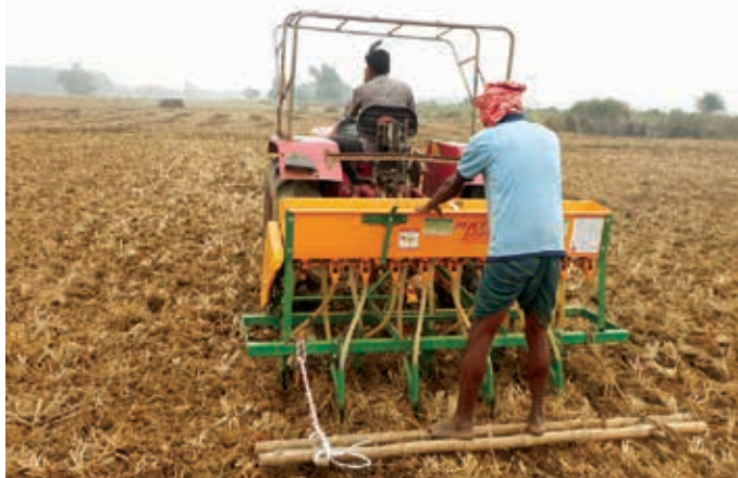
Mung bean sowing with seed-cum-fertilizer drill
