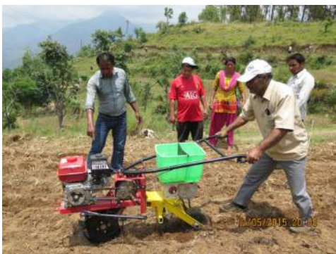
CHINESE POWERED SINGLE AND DOUBLE ROW DEDICATED MAIZE PLANTERS AND WEEDER AND FERTILIZER SIDE DRESSING
