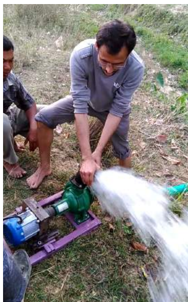
Bharat Paudel, testing the 48 V 850 watt DC motor powering a 3 inch centrifugal pump.
