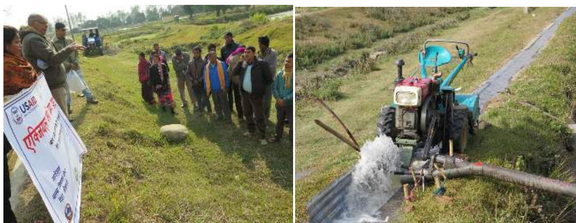
Axial flow pump demonstration in Fisheries Development Centre, Kailali
