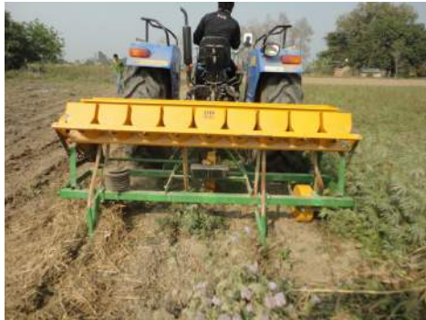
NATIONAL AGRO MULTI-CROP PLANTER USED FOR SEEDING THREE ROWS OF MAIZE IN ZERO-TILLED SOIL
