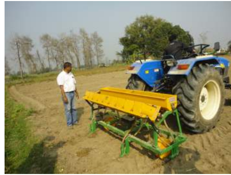
NATIONAL AGRO MULTI-CROP PLANTER USED FOR SEEDING TWO ROWS OF MAIZE IN A TILLED FIELD
