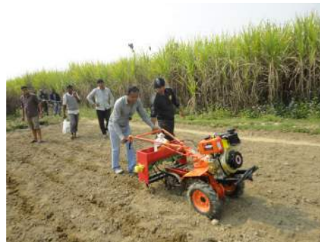
CHINESE 7-HORSEPOWER MINI-TILLER DRAWN FOUR-ROW PLANTER SEEDING MAIZE IN TWO ROWS
