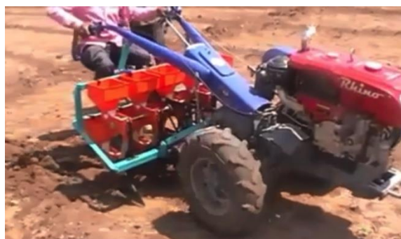
NEW DHARTI PROTOTYPE FOR LIGHTWEIGHT, ROAD TRANSPORTABLE, 2-WHEEL TRACTOR PLANTER-SEEDER THAT EMERGED FROM THE DESIGN SPRINT
