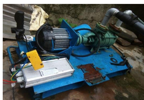
48 VOLT DC OFF-THE-SHELF E-RICKSHAW MOTOR WITH CONTROLLER ATTACHED TO OFF THE SHELF 2-INCH PUMP. TOTAL PRICE: UNDER US$ 300.
