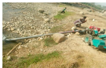
LOW LIFT AXIAL FLOW PUMP IRRIGATION INTO SMALL LINED CANAL VIA LOW COST LAY-FLAT PLASTIC DELIVERY PIPE. MAHADEVPUR, BANKE DISTRICT
