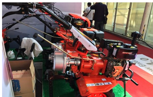
A 2 INCH OUTPUT DIAMETER IRRIGATION PUMP (SILVER COLOR) ATTACHED TO THE PTO SHAFT AT THE REAR OF A MINI TILLER ON DISPLAY IN SKT'S SHOWROOM BHAKTAPUR, NEPAL.
