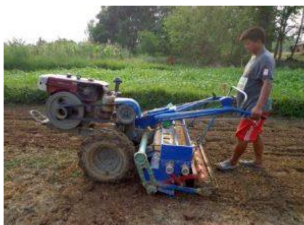
KARKA PUN WITH REDUCED TILL DRY DIRECT SEEDING RICE WITH A 2-WHEEL TRACTOR SINGLE PASS TILL DRILL ON HIS FARM IN CHHARBLOCK, BANKE DISTRICT, NEPAL.
