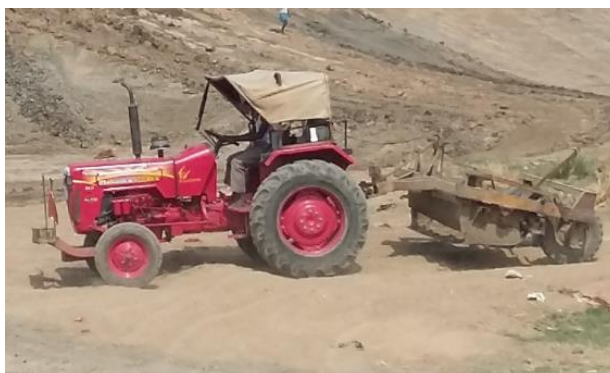
A TIPPING BUCKET: "NON LASER" LAND LEVELER BEING USED FOR POND EXCAVATION.
