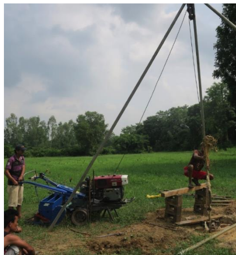
A 2WT BEING USED AS A WENCH IN LIFTING AND DROPPING A DRILL PIPE TO SPEED THE DRILLING OF SHALLOW TUBE WELLS. TOTAL COST OF THIS DRILLING RIG IS UNDER US$ 500, THE SAME PRICE AS A REAPER—HARVESTER ATTACHMENT.
