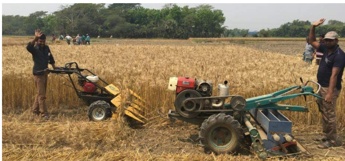
Machinery entrepreneurs harvesting wheat and establishing directly sown rice immediately after on the same field in Jessore Hub. These machinery options reduce turn-around time between crops and allow farmers to establish crops earlier, saving time, costs, and boosting yields while reducing production risks. Photo: T. Krupnik
