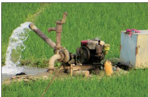
Shallow tube well irrigation pump driven by a diesel engine
