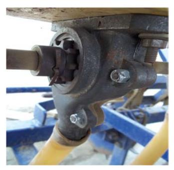
Figure 12. Flutted roller with shaft
