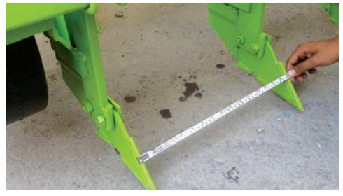
Figure 25. Distance between two alternate furrows
