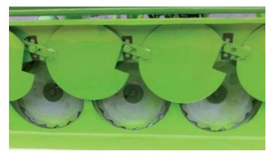
Figure 6. Inclined rotary plates (inside the seed box)
