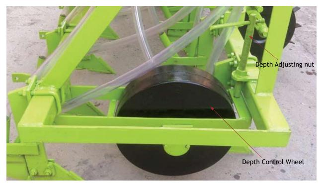
Figure 19. Depth control wheel and its adjustment
