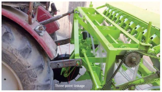
Figure 26. Hitching of machine through three-point linkage
