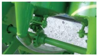
Figure 21. Power transmissions with Bevel gears
