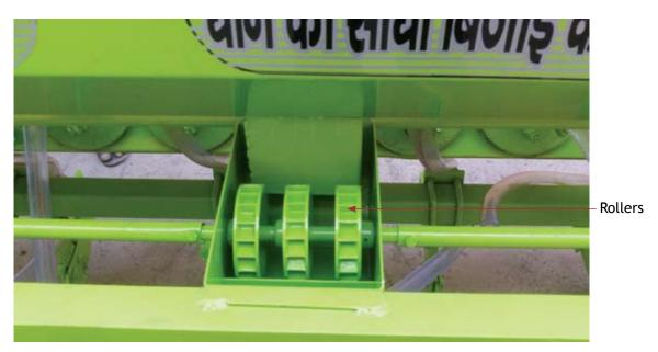
Figure 17. Cup/cell type roller
