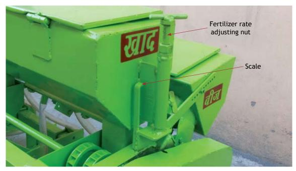
Figure 16. Fertilizer rate adjustment
