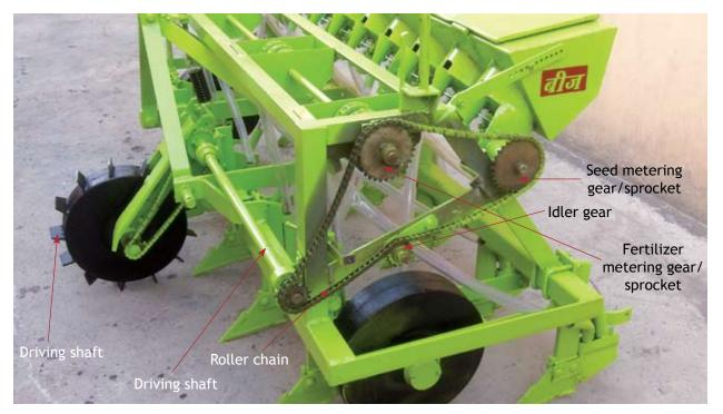
Figure 20. Power transmission unit and chain Mechanism
