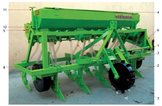
1. Frame, 2. Furrow openers, 3. Tynes, 4. Fertilizer box, 5. Seed box, 6. Chain and gear drives, 7. Drive wheel, 8. Depth control wheel, 9. Fertilizer delivery pipe, 10. Seed pipe, 11. Fertilizer rate adjusting nut, 12. Seed rate adjusting strip *Figure 1. Components of multi crop zero till planter*
