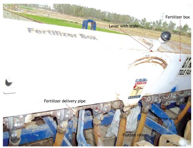
Figure 11. Fertilizer metering system
