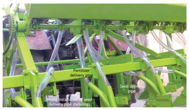
Figure 22. Seed and fertilizer delivery pipes
