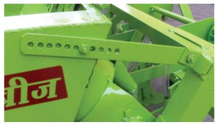
Figure 8. Seed metering strip with seed rate scale on it
