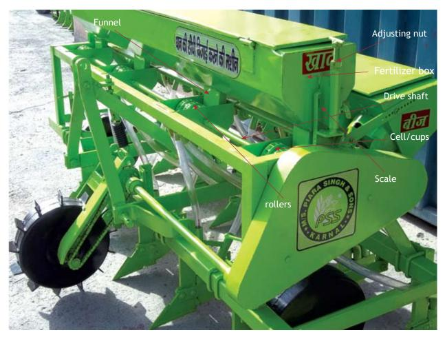
Figure 15. Fertilizer metering components
