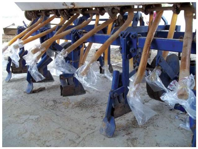
Figure 23. Seed and fertilizer calibration in laboratory
