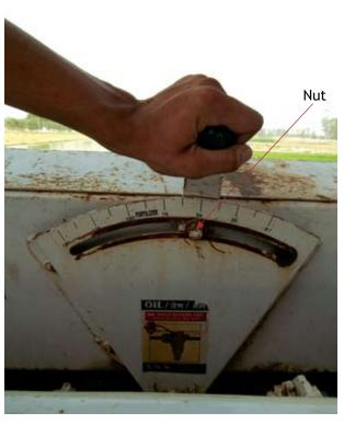
Figure 14. Fertilizer rate adjustment lever with scale and nut
