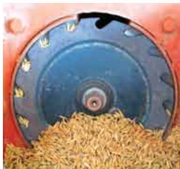
Inclined-plate (left) and fluted-roller (right) metering systems
