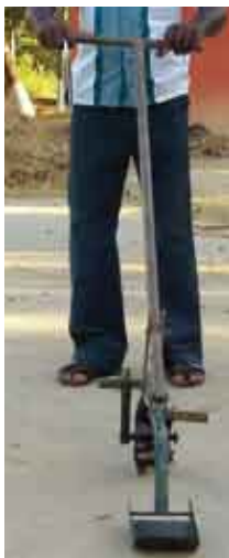
Hand-operated cono weeder for single-row and double-row weed control in DSR (front and side views)
