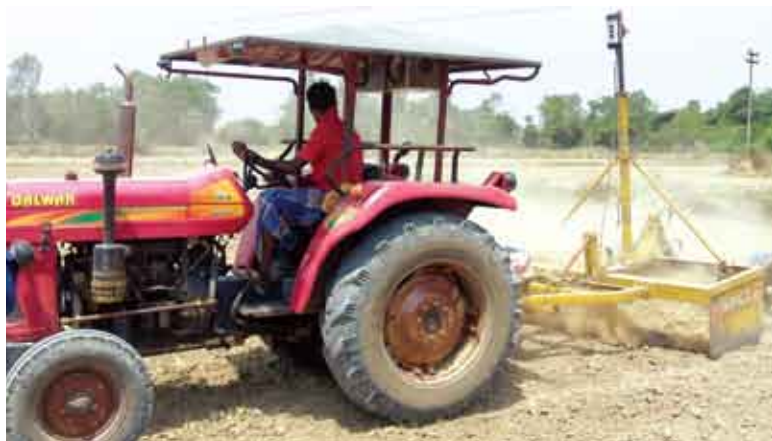
Land leveling using laser guidance
