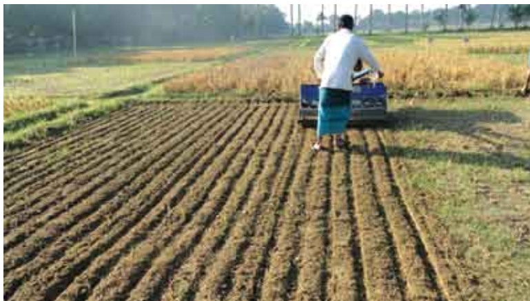
Seeding with strip tillage using a PTOS (“power tiller–operated seeder” – a seeder with tiller powered by a 2-wheel tractor)
