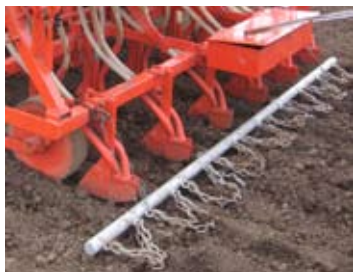
Coverage of seeds with soil using chains or flaps
