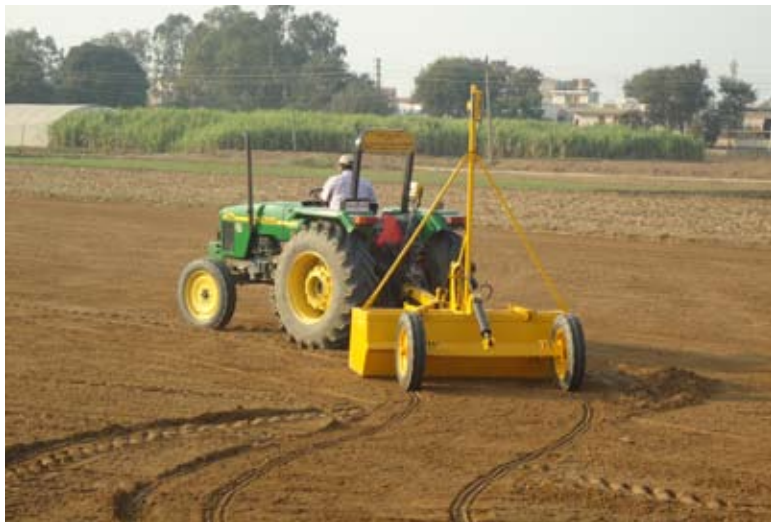
Land leveling using laser guidance
