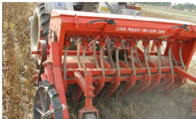
DSR being sown into residues using the Turbo Happy Seeder
