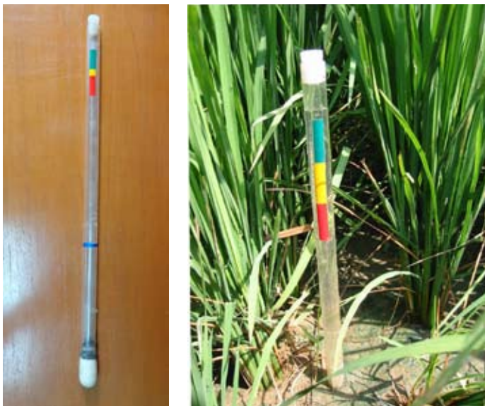
Farmer-friendly tensiometer for scheduling irrigation
