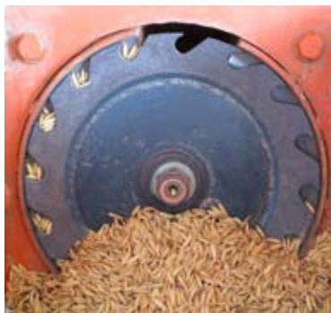
Inclined-plate (left) and fluted-roller (right) metering systems
