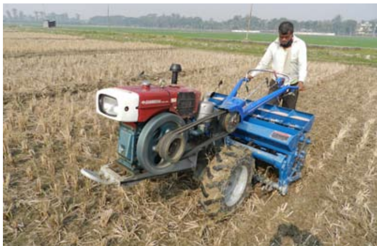
Crop being sown by a seed-cum-fertilizer drill with inclined-plate seeding mechanism, using full tillage, powered by a 2-wheel tractor. Tillage and seeding are done in a single pass.
