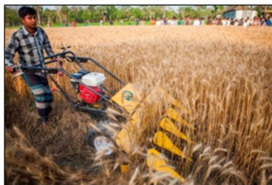
Above: A local service provider (LSP) demonstrates use of a self-propelled multi-crop reaper that reduces labor bottlenecks during harvest time. CSISA-MI partners with ACI to commercialize reapers in the FtF zone.
