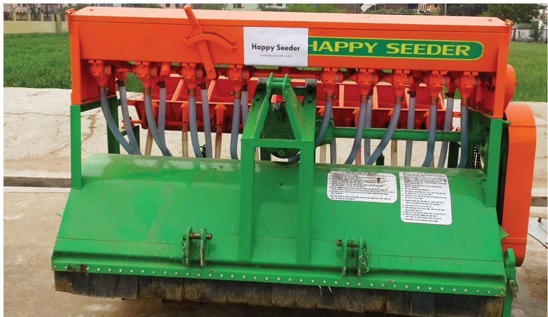
Photo 4: Happy seeder for direct drilling with 100 percent residue load.
