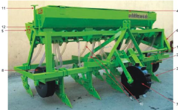
1. Frame, 2. Furrow openers, 3. Tynes, 4. Fertilizer box, 5. Seed box, 6. Chain and gear drives, 7. Drive wheel, 8. Depth control wheel, 9. Fertilizer delivery pipe, 10. Seed pipe, 11. Fertilizer rate adjusting nut, 12. Seed rate adjusting strip
