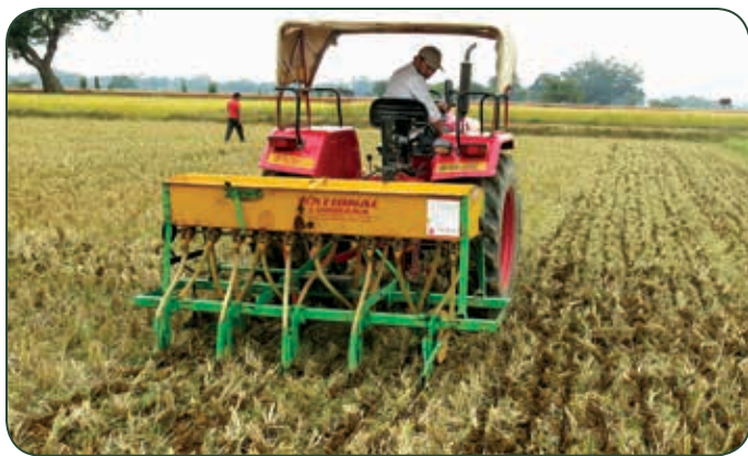
Sowing of toria using seed drill in ZT
