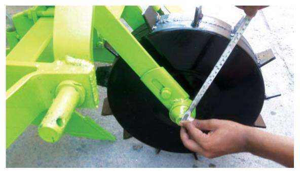
Figure 24. Diameter of drive Wheel
