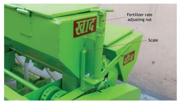
Figure 16. Fertilizer rate adjustment
