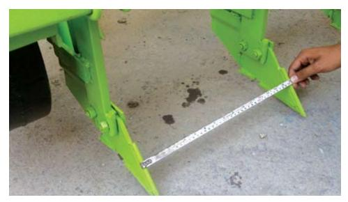
Figure 25. Distance between two alternate furrows
