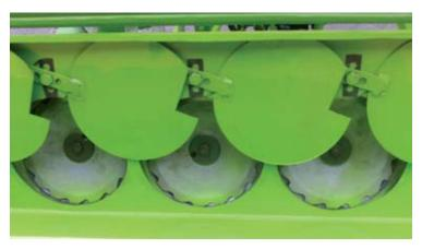
Figure 6. Inclined rotary plates (inside the seed box)
