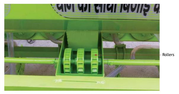
Figure 17. Cup/cell type roller
