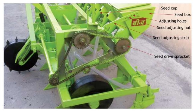
Figure 5. Seed metering mechanism and its components
