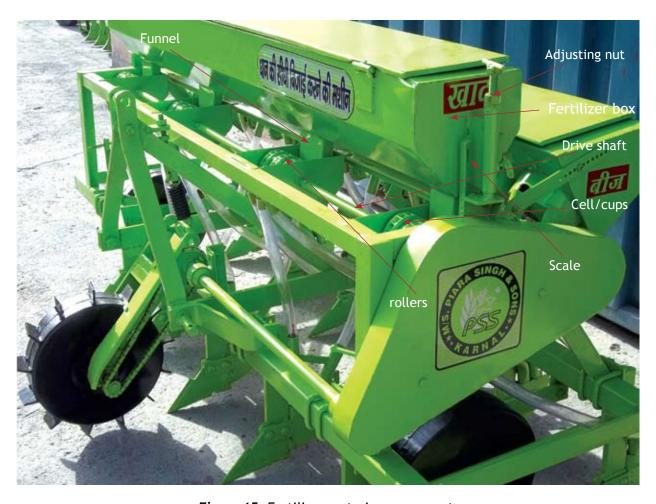
Figure 15. Fertilizer metering components
