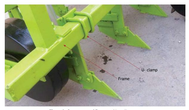
Figure 2. Components of Frame and its adjustment
