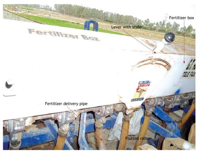
Figure 11. Fertilizer metering system
