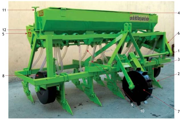
1. Frame, 2. Furrow openers, 3. Tynes, 4. Fertilizer box, 5. Seed box, 6. Chain and gear drives, 7. Drive wheel, 8. Depth control wheel, 9. Fertilizer delivery pipe, 10. Seed pipe, 11. Fertilizer rate adjusting nut, 12. Seed rate adjusting strip
