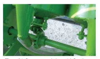
Figure 21. Power transmissions with Bevel gears
