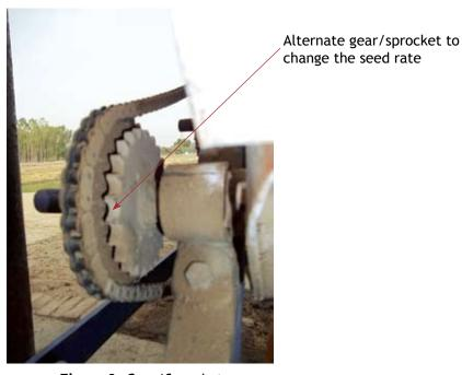
Figure 9. Gear/Sprocket
